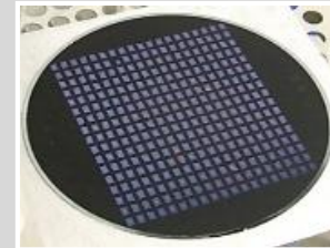
FO-WLP die first, RDL first, multi-strata, organic, silicon, glass substrates
